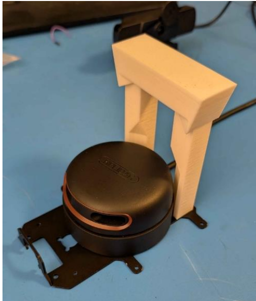
Figure 45: Physical Camera Mount and Lidar Fit Test
