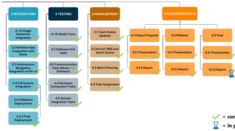
Figure 52: WBS Integration, Testing, Management & Documentation Stages
