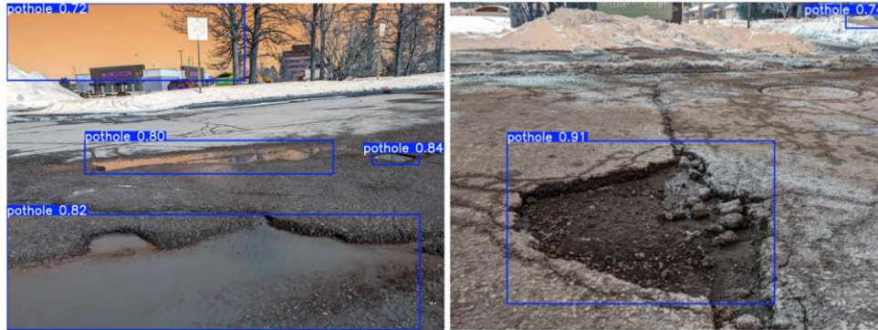
Figure 22: Examples of False Positive Detections
